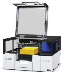
Print on 3D objects, up to 70 mm thickness
